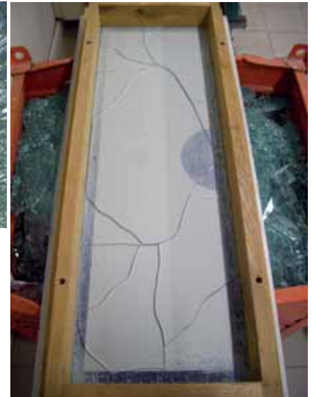
Figure 1 Fragmentation pattern in thermally toughened safety glass (a) and in heat strengthened glass (b).
